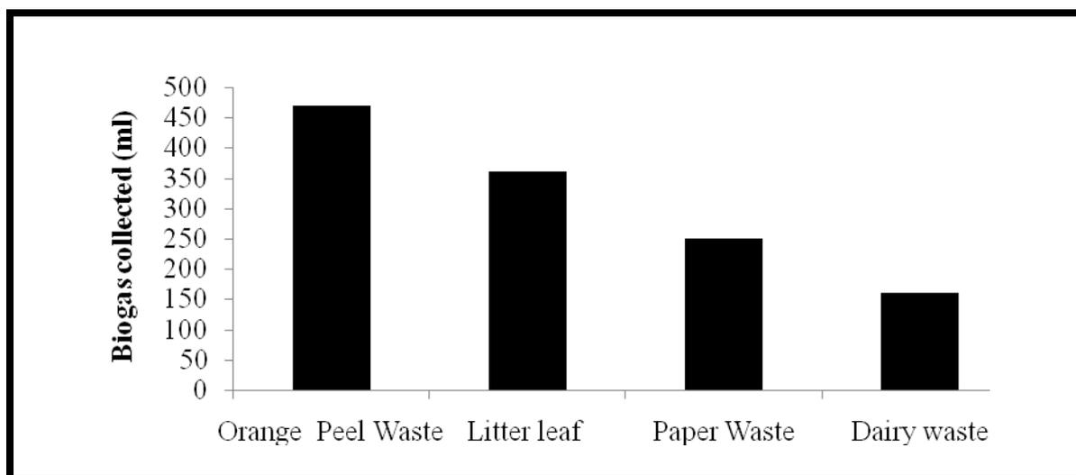
**Figure 2: Effect of different wastes on Biogas Production**
